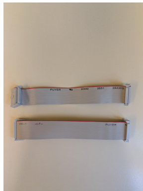
Figure 6: IDC ribbon cables.
